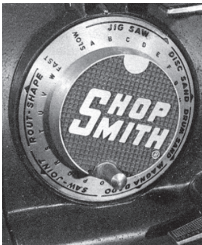
Figure 1-33. The speed dial is letter calibrated through an rpm range of 700 to 5200. Caution: Turn the dial only when the motor is running. When an operation is complete, always turn the dial to 'Slow' before shutting off the Mark V.
