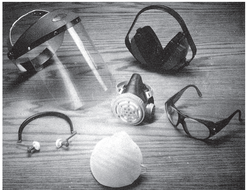
Figure 1-31. These are devices that protect you from eye, ear, face and respiratory injuries. Their cost is slight when you consider the protection they afford. And they can be used for activities in addition to power tool work.
